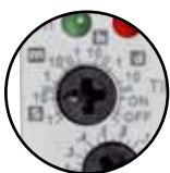
Rough time setting - IMPULS time setting in range 0.1 .. 10 days
