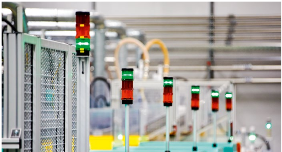
Signal towers with tube mounting
