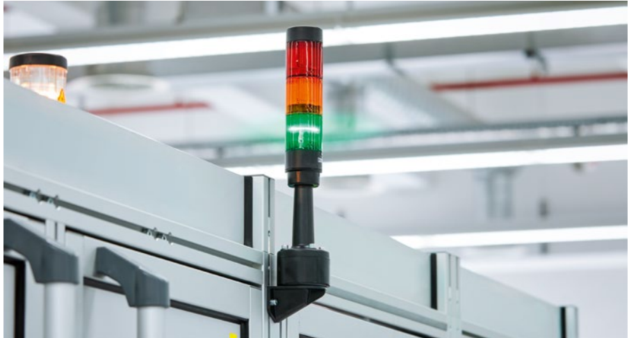
Signal tower assembled with three color calottes
