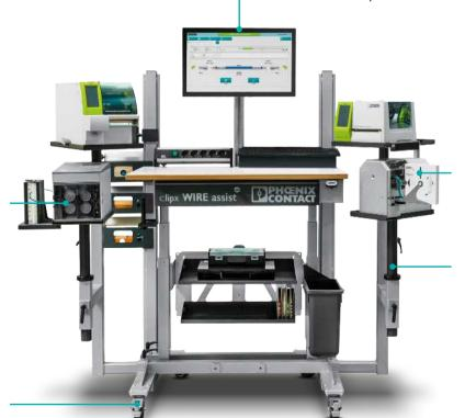
Proven automatic tools, such as the CF 3000 and the WF 1000, as well as printing systems of the THERMOMARK series ensure process-reliable and efficient wire processing.
